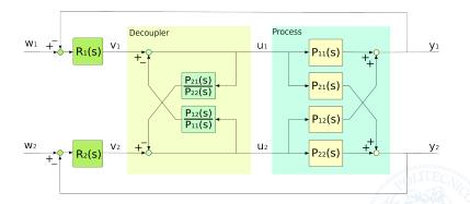
• The two controllers  $R_1(s)$  and  $R_2(s)$  are designed with known SISO techniques, as if one were dealing with two independent processes having transfer function  $P_{11}(s)$  and  $P_{22}(s)$ , respectively
