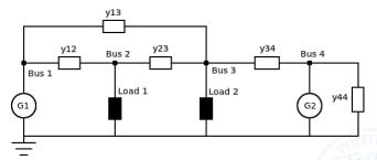
• Remove all generators and loads, denote by <u>V</u><sub>i</sub> the voltage at the *i*-th bus, inject in each bus a current <u>L</u><sub>i</sub>, write the nodal equations (KCL), and solve for the injected nodal currents. You have three minutes, then we do it together.
